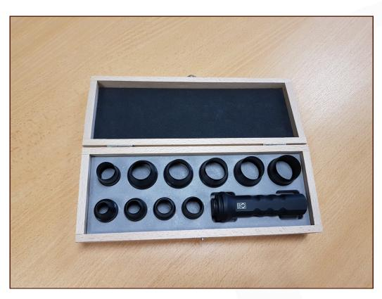
Handle weight + hollow punch : env. 210 gr Dimensions : 25 x 27 mm and 35 x 32 mm Weight : 950 gr
